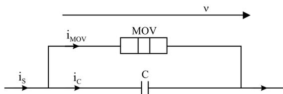
Fig. 2. Equivalent circuit of TCSC when thyristors are in block state.
