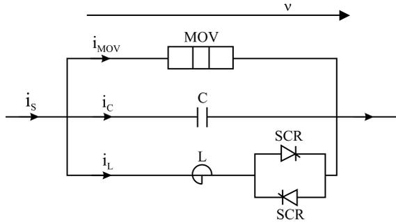
Fig. 1. The main circuit of TCSC.
