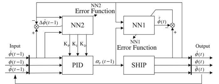
Fig. 2. The control system scheme for self-tuning neural network PID controller
