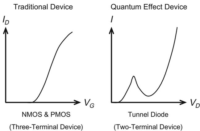
Fig. 1. Nonlinear current voltage characteristics of MOSFET and tunnel diode.
