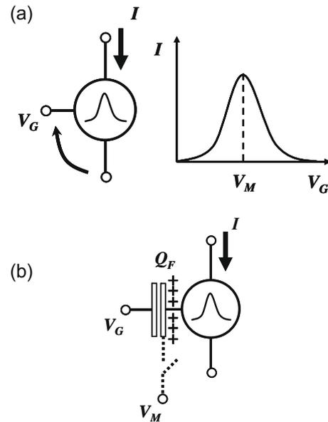
Fig. 3. Quantum-effect device having resonance-type  $I-V$  characteristics.
