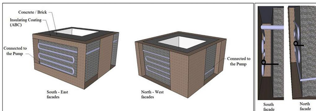
Fig. 1. Active embedded water pipe wall loop system.
