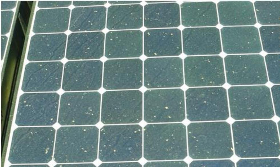
Fig. 1 Dust accumulation on PV panel in UCSD.
