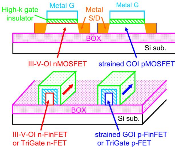
Fig. 1. Ultimate CMOS device structure composed of III-V nMOSFET and Ge pMOSFET.
