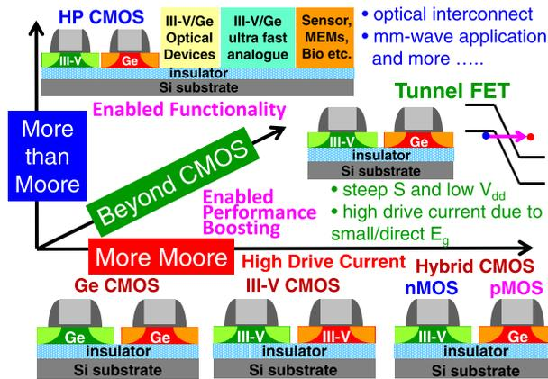
Fig. 2. Possible evolution scenario for III-V/Ge devices on Si platform through heterogeneous integration.
