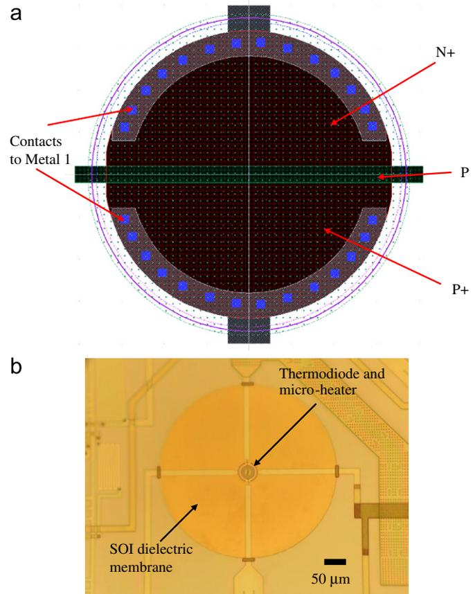
Fig. 2. (a). Cadence layout of the SOI p+/p/n+ thermodiode with diameter of 34 μm. (b). The optical micrograph of a fabricated micro-hotplate with SOI thermodiode temperature sensor embedded under the hotplate, within the oxide membrane.
