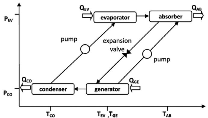
Fig. 1. Schematic diagram of a basic AHT.
