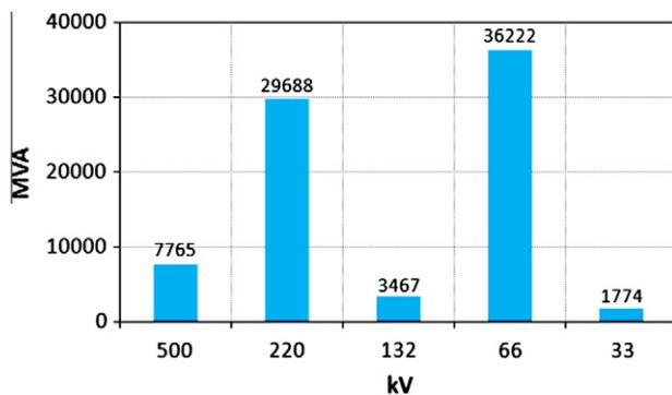
Fig. 1. The EETC's total Transformers Capacities in 2008–2009.
