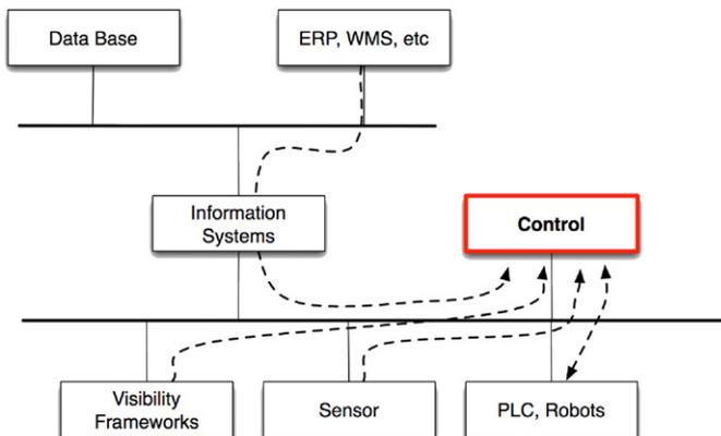
Fig. 1. Current information flow in the control systems.
