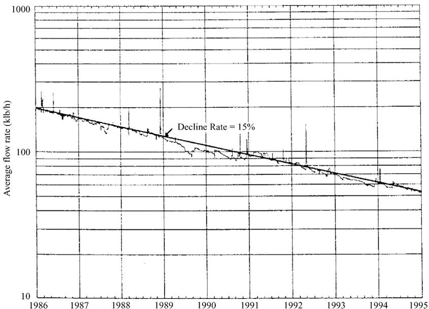
Fig. 1. Example of 150% production decrease over 10 years in the steam reservoir at Calistoga, USA (average daily flow rate versus time; from Sanyal et al., 2000).
