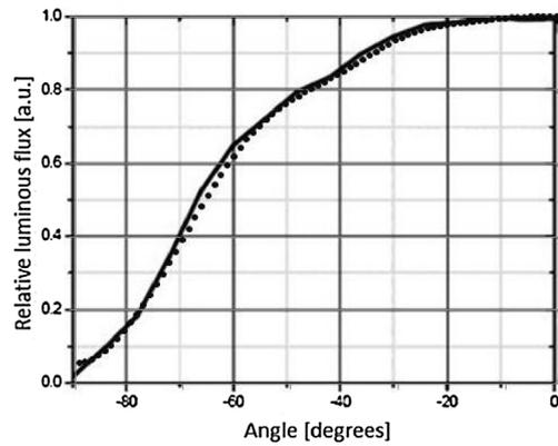
Fig. 3. LED emission profile in Cartesian coordinates, showing its forward directionality. Solid line: from LED data sheet. Dots: realistic directional model of the LED emission.
