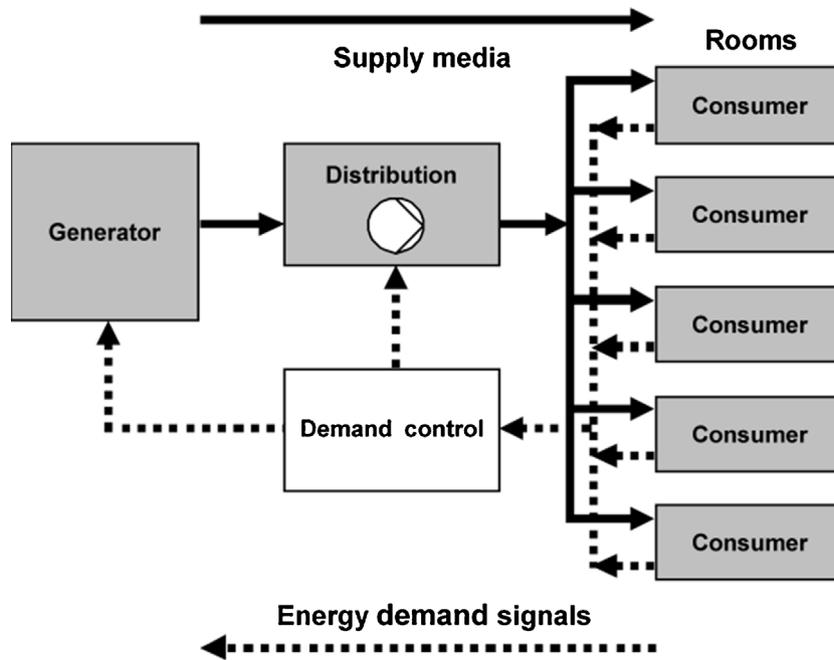
Fig. 1. Demand control according to EN 15232.
