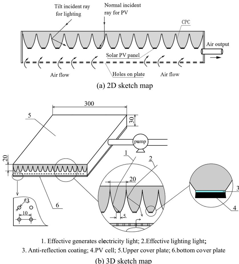
Fig. 1. The working principle of the PV/T/D device.
