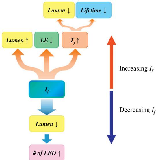
Fig. 1. Effect of  $I_f$  on performance of LED-based luminaire.
