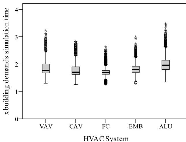
Fig. 2. Simulation time ratio: detailed HVAC system model vs. building heating/cooling demand.
