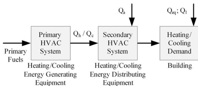
Fig. 1. Energy flow of principal HVAC system within buildings.
