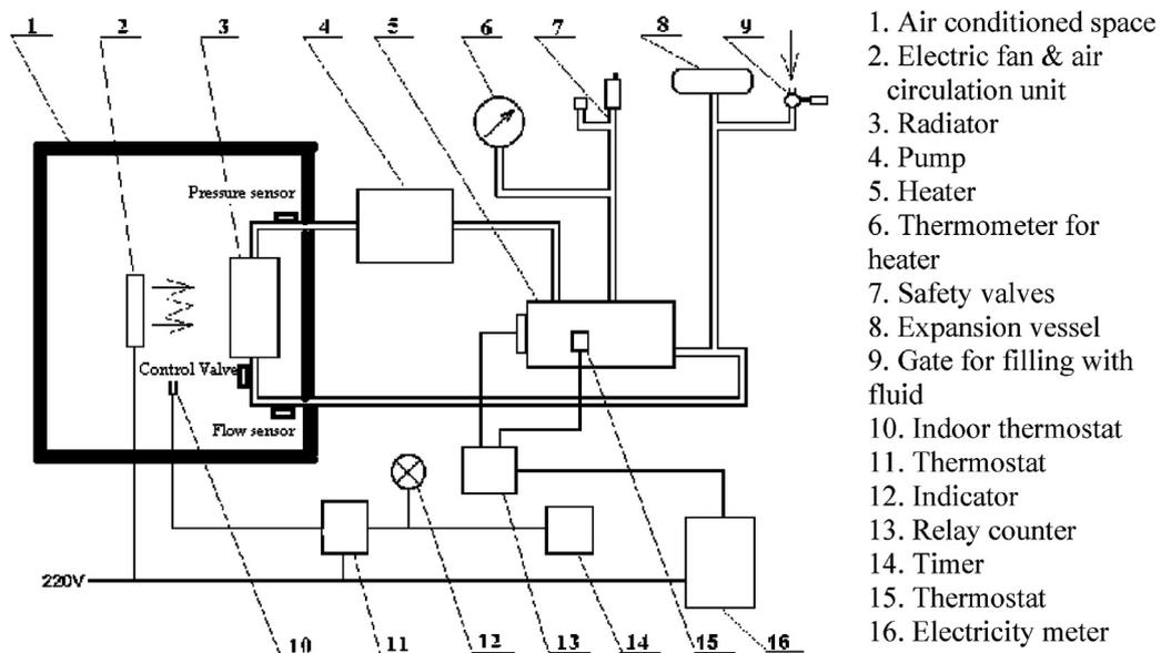
Fig. 1. Block diagram of the small scale central heating system.
