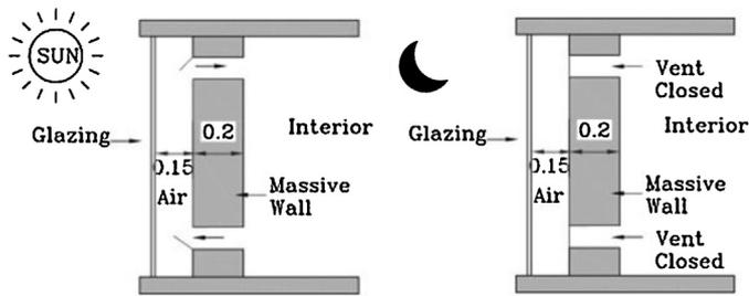
Fig. 1. Typical structure form of the Trombe wall.
