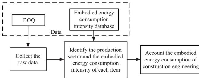
Fig. 1. Accounting procedure for energy consumption of construction engineering.
