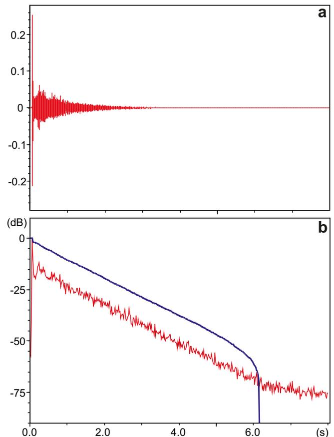
Fig. 1. (a) Room impulse response, RIR; and (b) energy time curve, ETC, with the Schroeder's integral (thick line) calculated with noise compensation. (All measured at the receiver point R3, for source S1, filtered at 1 kHz in the Cathedral of Malaga).
