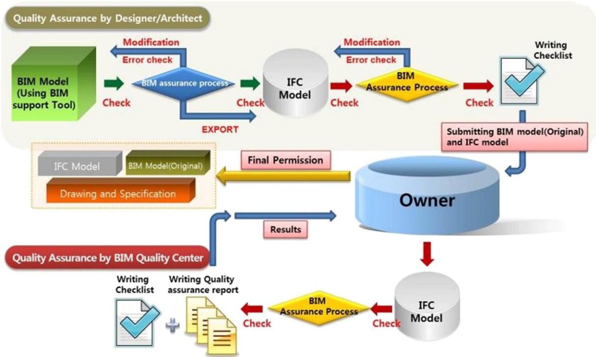
Fig. 1. BIM-based quality assurance process plan in Korea [12].
