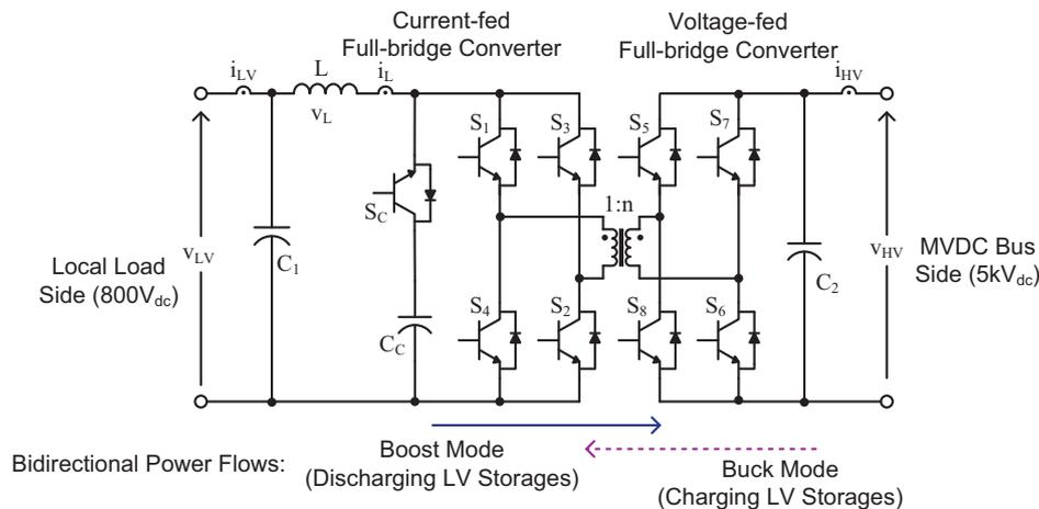
Fig. 2. Circuit diagram of bi-directional DC-DC Converter.
