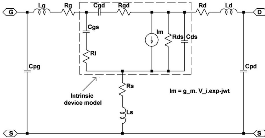
Fig. 1. Schematic diagram of MESFET small signal model.
