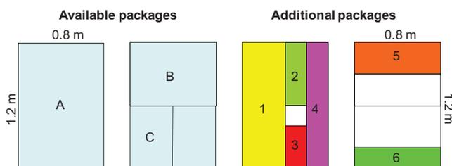
Fig. 1. Illustration of containers (Top View) used in this project with the 'Big Box' and two smaller sized packages currently in use on the left side (identified A, B, and C). To the right additional proposed 'narrow bin' containers (numbered 1–6) are positioned as designed to fit on the same 'Europallet' footprint as the Big Box.
