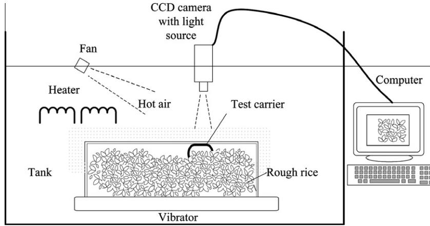
Fig. 1. The rice dryer and inspection device for the rough rice.
