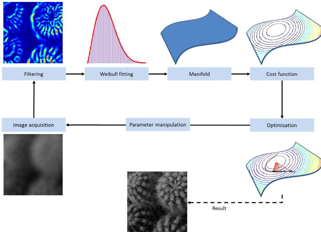
Fig. 1. An outline of the main components of our image processing framework, illustrating the autofocus problem. The starting point is the image acquisition step.
