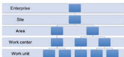
Fig. 1. Hierarchical levels according to ISO 22400-2:2014
