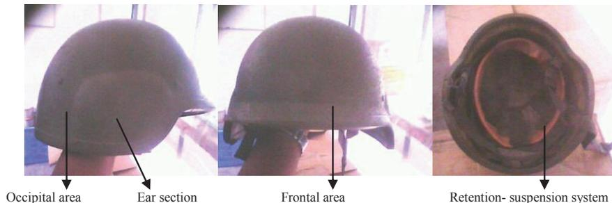
Fig. 2. The main design features of a PASGT helmet.
