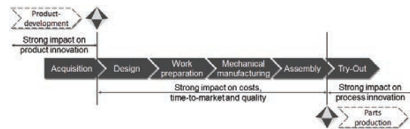
Figure 1 Present position of the tool maker's order fulfilment process within the customer's value chain [13]
