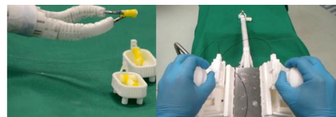
Fig. 1. Prototype of the multi-arm snake-like manipulator, fabricated by selective laser sintering of a biocompatible polyamide
