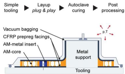
Fig. 1. Hand layup process route combining additive manufacturing and FRP.
