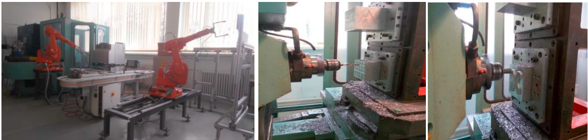
Fig. 1. Example of (a) Flexible manufacturing cell from Faculty of Managerial and Technological Engineering, University of Oradea, (b) Drilling processing, (c) Contour processing
