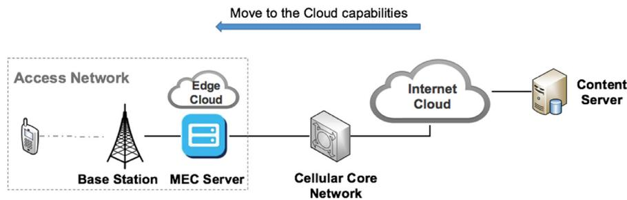
Fig. 2. Network system for the mobile edge cloud [7].
