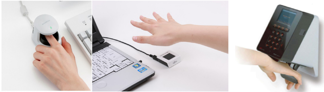
Fig. 1. Left: Hitachi finger vein scanner. Center: Fujitsu palm vein scanner. Right : Techsphere VP-II dorsal vein scanner [23–25].
