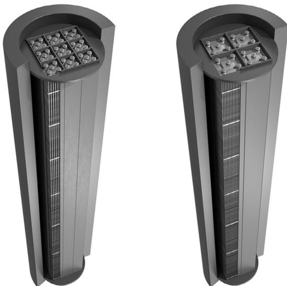
Fig. 1. Cross section of a BWR (left) and PWR (right) final disposal canister (Nagra, 2003).
