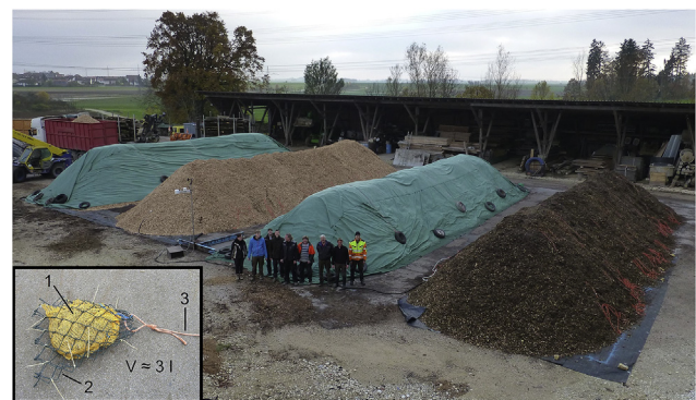
Fig. 1. Storage site with the four wood chip piles after the start of the winter trial. Left: two ERC piles, right: two FRC piles, each assortment with and without rain protection (fleece). FRC: forest residue chips, ERC: energy roundwood chips. In the black frame: Balance bag for retrieving wood chip samples from the piles, consisting of a net bag with wood chip sample (1), wire mesh for stabilization (2) and a drag rope (3).
