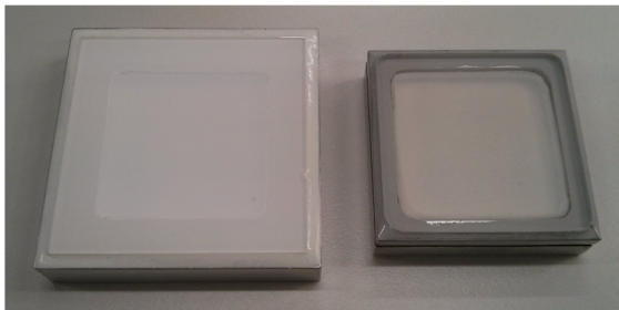
Fig. 2. Scintillator crystals of 25.8 \times 25.8 \times 5 \text{ mm}^3 active volume: \text{LaBr}_3 from Saint Gobain (left) and \text{CeBr}_3 from Hellma Materials (right).
