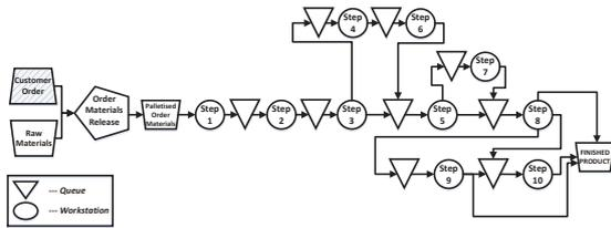
Figure 1. Process Flow
