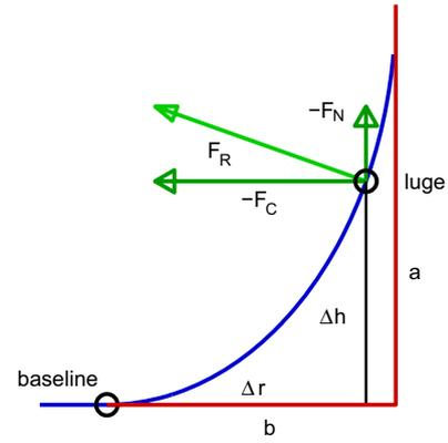
Fig. 2. Forces acting on the luge. The position of the luge is given by that point of the quarter ellipse for which the surface reaction force  $F_R$  is normal to the ellipse. Note, the cross section shown in the diagram is normal to the baseline, hence, inclined by the angle  $\alpha_0$  to the vertical.
